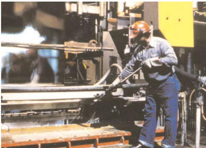
▲As metal comes out of the zinc pot on the way to the cooling tower, the coating thickness is regulated by the use of “air knives,” or pneumatic squeegees.
