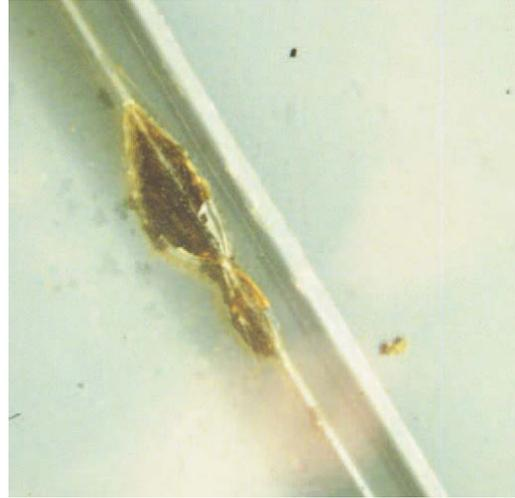
The view down into a seam area shows corrosion that began on the inside and worked its way out.
