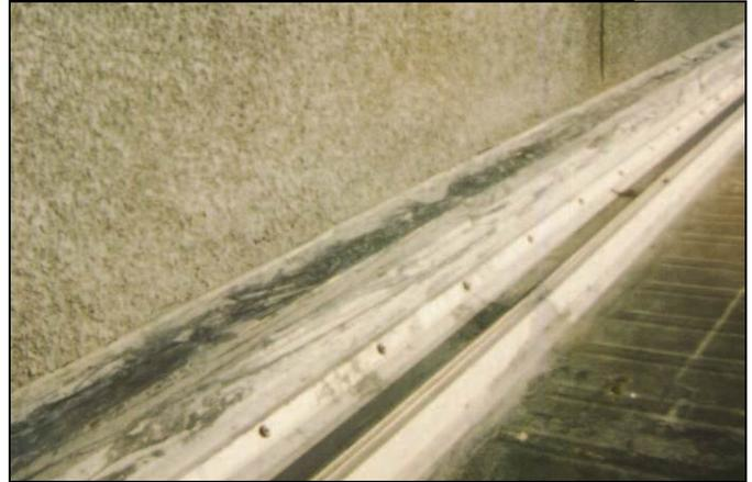
(Top) Improper storage and/or transit of Galvalume panels can result in damage from trapped moisture.
