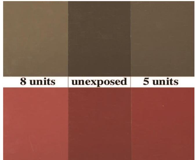
▲ Color change (fade) is measured in NBS Units or ΔE Hunter Units. One unit is the smallest degree of fade detectable to a trained eye. Premium paint warranties usually limit fade to 5 units. *Image courtesy of Metal Roof Advisory Group, Ltd.*
