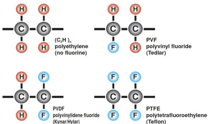
▲ This shows the molecular structure of fluoropolymer coatings, their respective trade names and a comparison to a polyethylene molecule. These polymers have similar properties derived from their atomic structure and fluorine bonds. *Image courtesy of Metal Roof Advisory Group, Ltd.*
