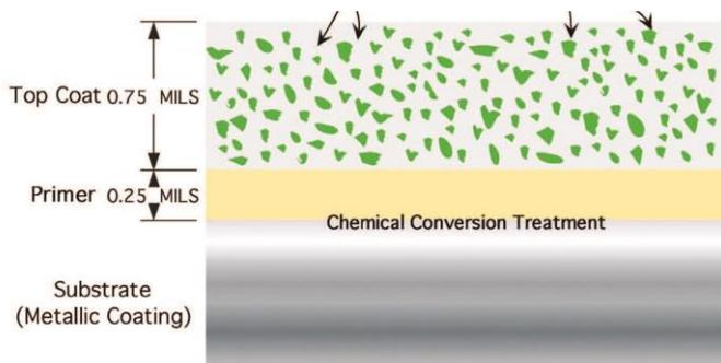
▲ Most popular architectural paint finishes are two-coat systems, resulting in a dry film thickness of about 1.0 mil. *Image courtesy of Metal Roof Advisory Group, Ltd., Colorado Springs, CO.*
