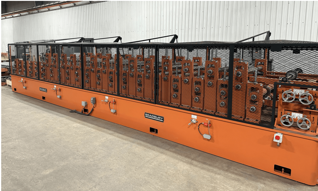
Figure 2. In-line roll former Image courtesy of McElroy Metals
