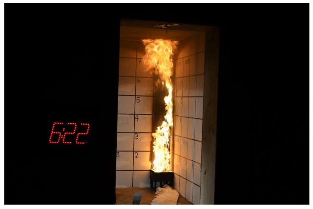
NFPA 286 Fire Test Flame, at 160 kW
