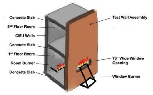
The test wall assembly specimen must be at least 17.5 ft. high by 13.3 ft. wide.
