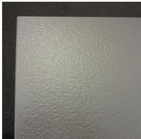
**Photo #3:** Typical embossing for IMPs, viewing distance 18 inches.
